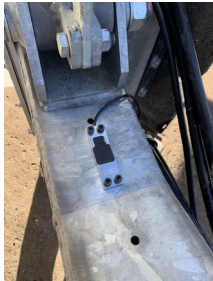
Fig. 10 – Strain gauge sensor on the drawbar tube
