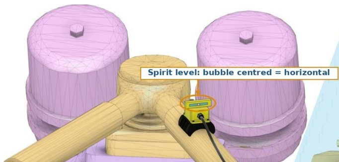
Fig. 9 – Checking the horizontal alignment with a spirit level
