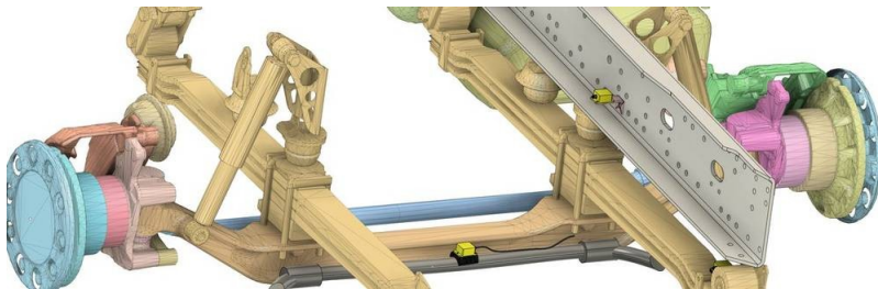
Fig. 3 – Angle sensors S0 (frame) and S1 (anti-roll bar)
